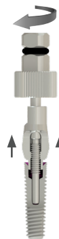
The tool continues rotating, it will disengage the con- nection and gently lift the abutment.
